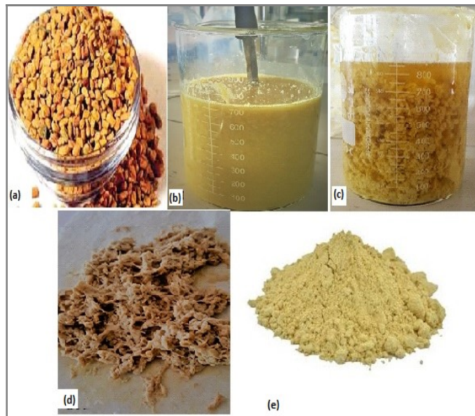
Fig 1. Figure shows (a) Fenugreek seeds, b) Soaked fenugreek powder for 5 h and boiled for 2 h, c) Precipitated fenugreek seed mucilage after adding ethanol, d) Extracted fenugreek seed mucilage after filtration, and e) Dried and grounded fenugreek mucilage powder after passing through sieve No. # 60 mesh.
